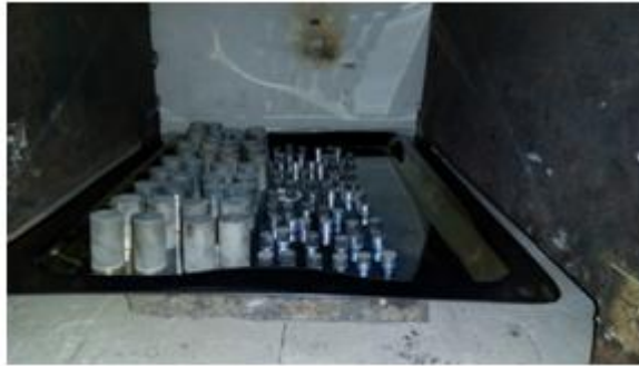
Figure 2. Specimens kept inside sintering furnace
